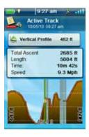
The Altimeter Screen displays detailed elevation information using the GPS signal. The area on the graph can be expanded by Selecting the icon in the lower right corner and defining the area to be used. Also a line can be moved along the graph to pinpoint an exact point on the graph and display detailed information on that point.
