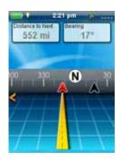
The Road screen displays a graphical road with a strip compass above the road. This compass displays your heading and your heading's relation to the sun, moon and your destination (black arrow) when they are within 50 degrees on either side of your heading. The data fields at the top of the display are customizable (see *Customizing the Data Fields*).
