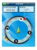
The Compass screen displays a recognizable compass that can be used to display your heading and your heading's relation to the sun, moon and your destination (black arrow). The data fields at the top of the display are customizable (see *Customizing the Data Fields*). The graphic displayed that is used for the compass is customizable as well.
